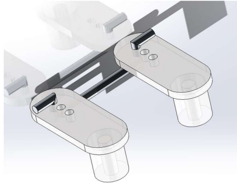
Figure 41: Image of the servo linkage that will control steering
